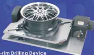
Car-rim Drilling Device (Car Drill Air-inlet at 80°)
